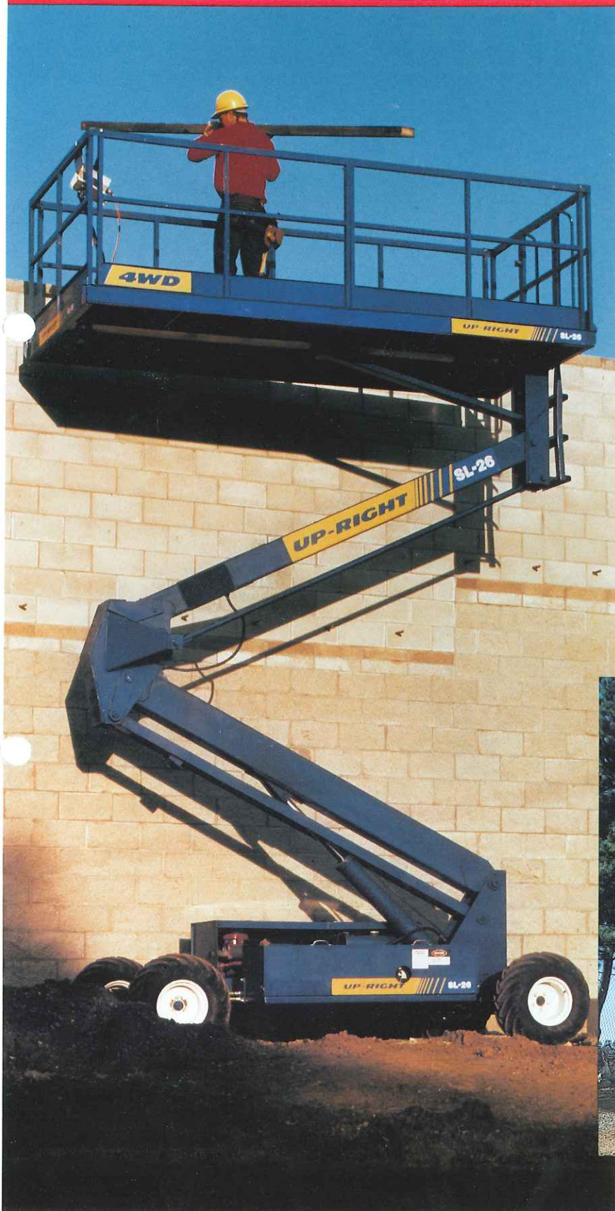
Oscillating front axle for optimum rough terrain capability.
