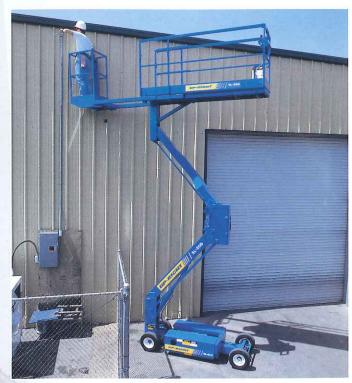
Optional 6 ft. cantilever deck provides 8 ft. (2.44 m) of overreach.
