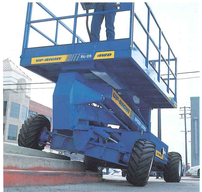
Oscillating front axle for optimum rough terrain capability.
