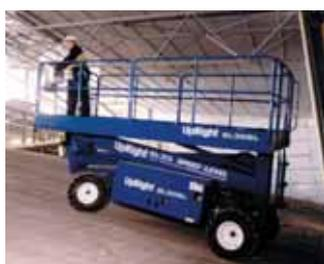
All models have oscillating axles to keep drive wheels in contact with uneven ground and have high levels of gradeability for tough sites and loading ramps.
