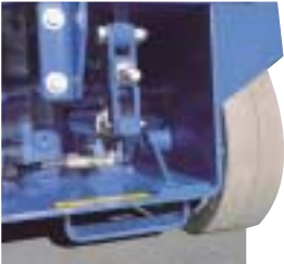
Non-marking tyres are fitted as standard to protect floor finishes.
