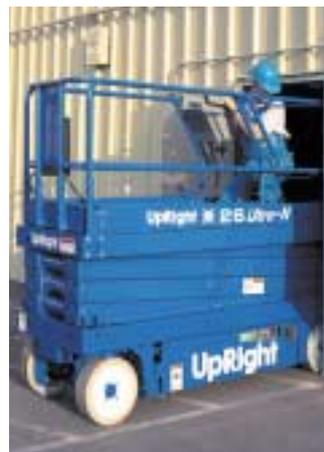
Quick retract guard rails and only 825mm (32.5in.) wide the X26 Ultra-N will pass through a single standard doorway.
