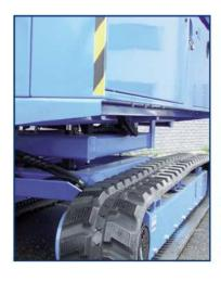
300mm tracks - ideal for rough terrain applications and where low ground bearing pressure is
