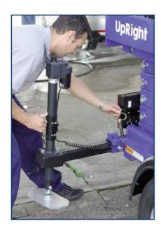
Quick and easy to set up outriggers pull out and lock into place. One button to autolevel the machine ready for use.
