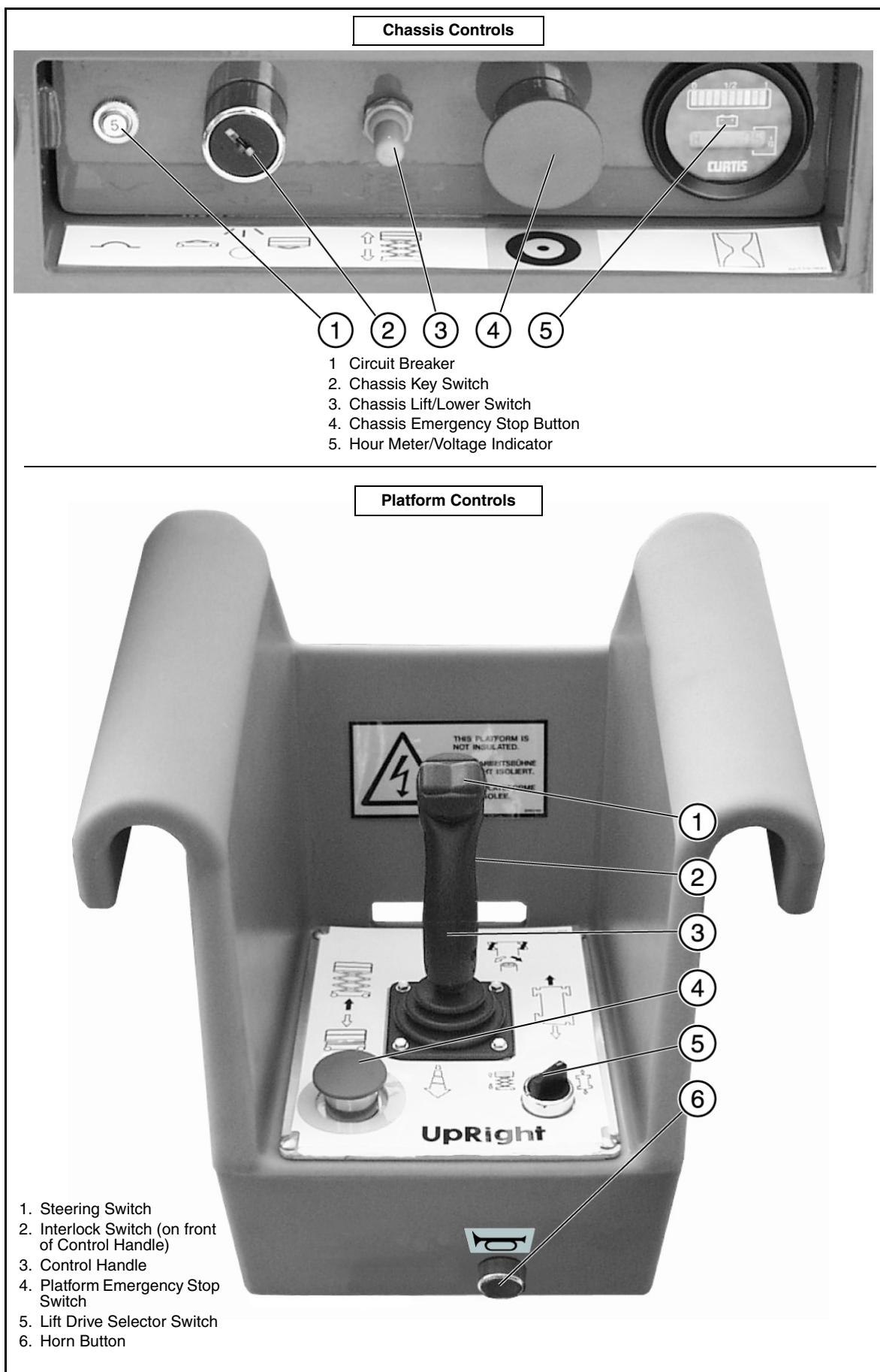
Figure 2: Controls and Indicators
