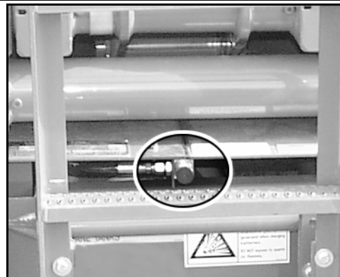
Figure 3: Emergency Lowering Valve Knob
