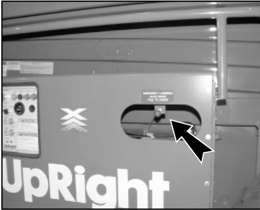
Figure 5: Emergency Lowering Valve Knob (XRT27)
