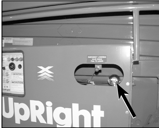
Figure 4: Emergency Lowering Valve Knob (XRT27)
