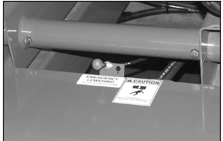
Figure 5: Emergency Lowering Knob, LX31 and LX41
