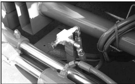
Figure 1: Emergency Lowering Valve
