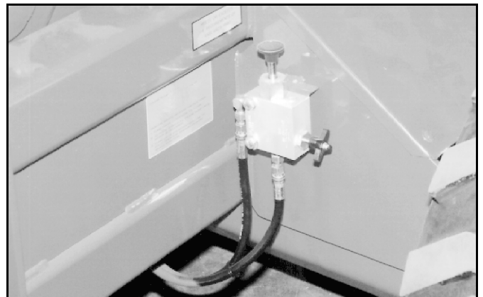
Figure 2: Parking Brake Release Pump
