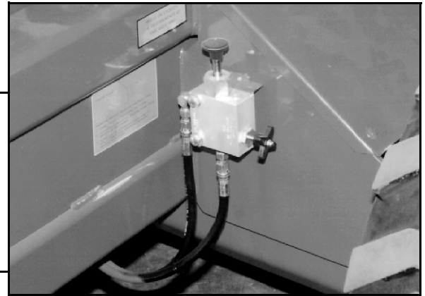
Figure 6: Parking Brake Release Pump
