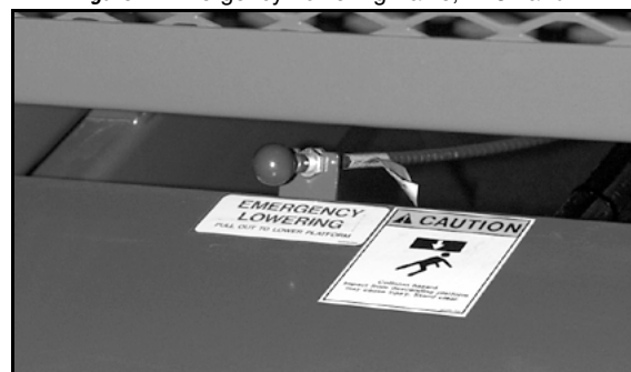
Figure 4: Emergency Lowering Valve, LX31 and LX41
