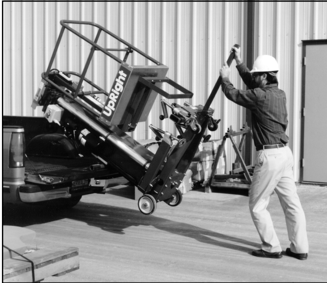
Figure 8: Tilting machine onto or off of a vehicle
