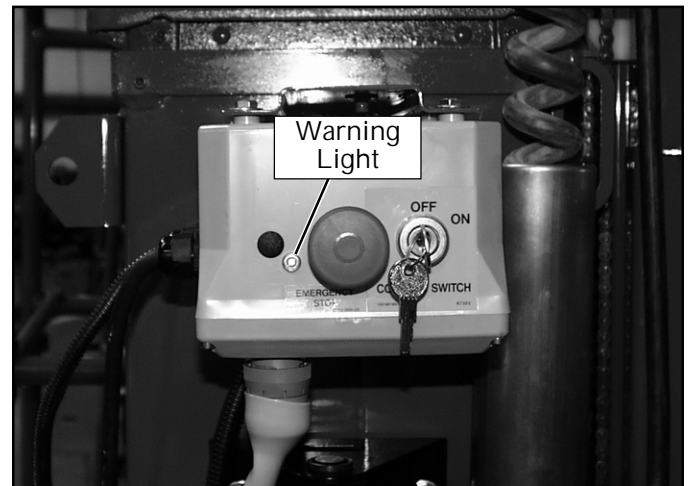
Figure 4: Warning light shines when batteries for optional auxiliary platform lowering circuit are low.
