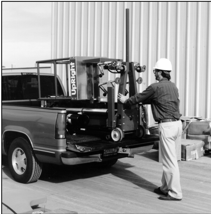
Figure 9: Pushing machine into transport position
