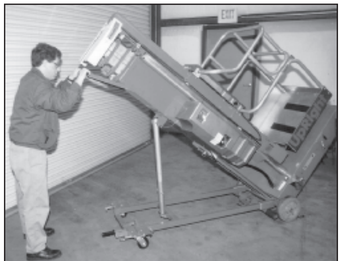
Figure 10: Compressing cylinder assembly
