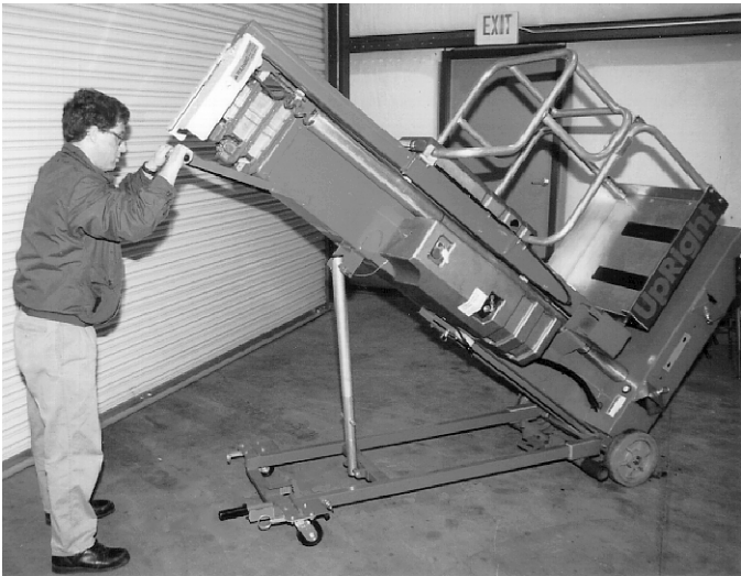
Compressing the Cylinder Assembly
