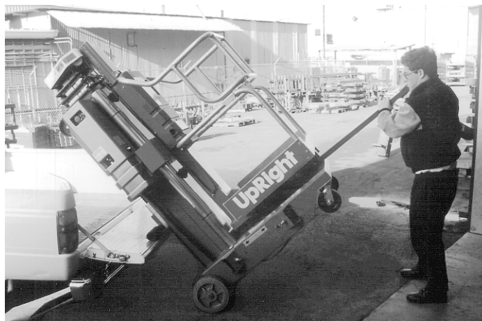
Tilting the Machine Onto or Off of a Vehicle
