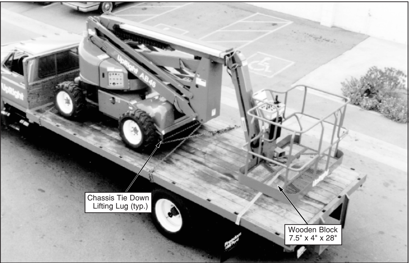
Figure 6: Securing the Machine for Transportation
