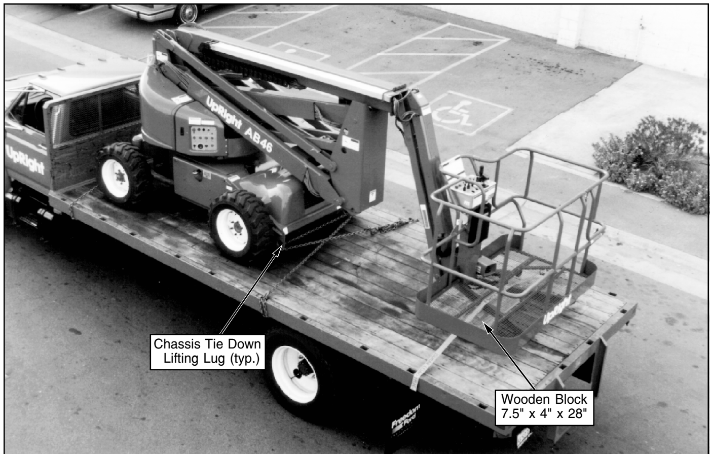
Figure 6: Securing the Machine for Transportation
