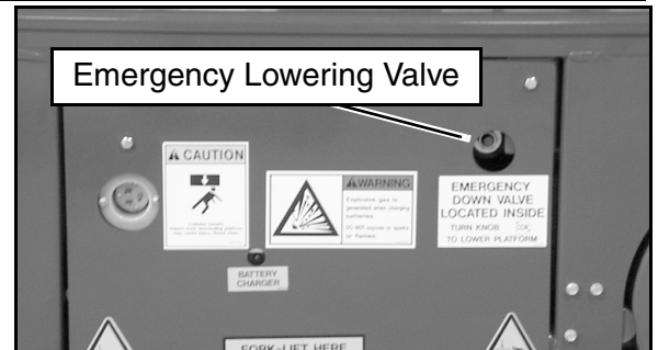
Figure 4: Emergency Lowering Valve
