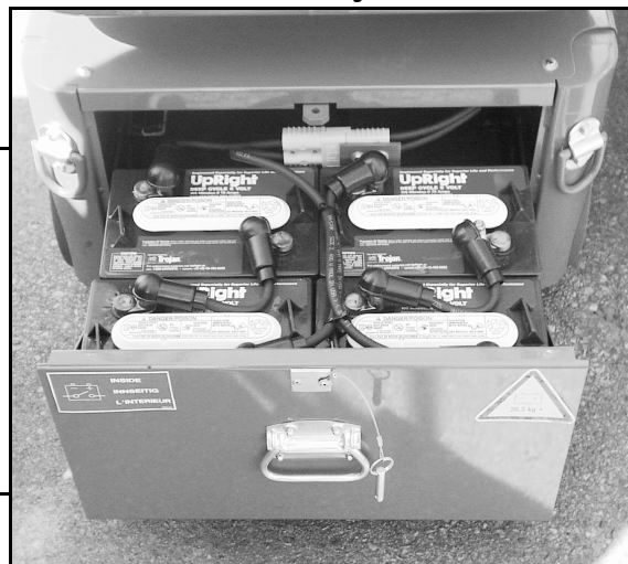
Figure 9: Access to Batteries
