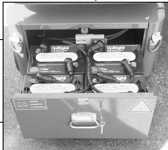
Figure 9: Access to Batteries
