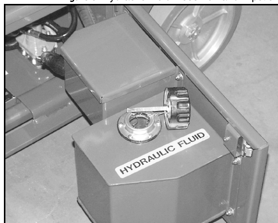
Figure 8: Hydraulic Fluid Reservoir and Dipstick
