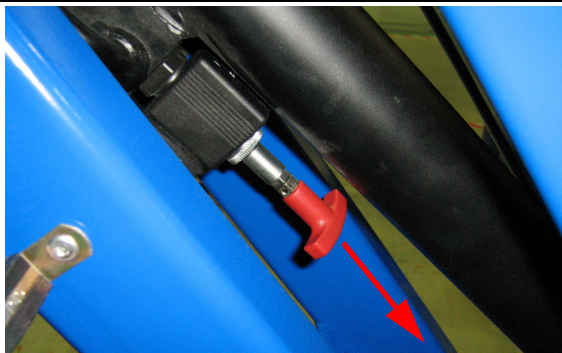
Figure 9: Emergency Lowering - Jib Valve
