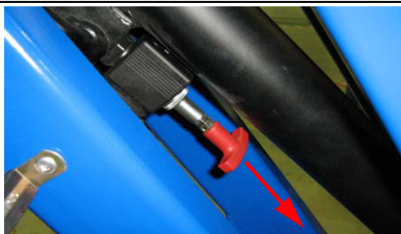
Figure 9: Emergency Lowering - Jib Valve
