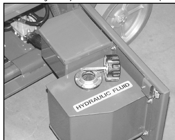
Figure 8: Hydraulic Fluid Reservoir and Dipstick
