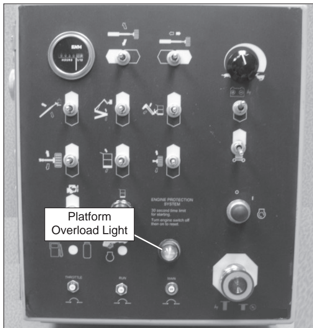
Figure 4.7 – Lower Control Panel
