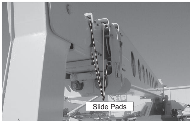
Figure 7.18 – Slide Pads at Tip End of Boom
