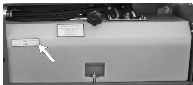
Figure 4.4 - Hydraulic Oil Level
