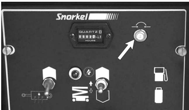
Figure 5.4 - Main Circuit Breaker
