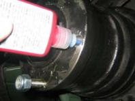
Loctite 648 Loctite cleaning solvent Degreasing wipes
