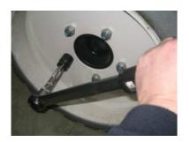
Tools: M22 socket Wrench extension bar Torque wrench set 145 N/M 2.5 Ton Jack
