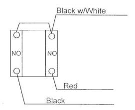
Back of fuel selector switch Rewired with new contact block
