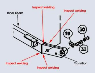
"Inspect the machine thoroughly for cracked welds and structural damage, loose or missing hardware, hydraulic leaks, damaged control cable and loose wire connections."
