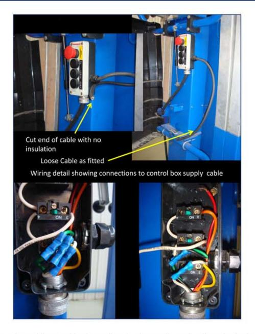
In addition to carrying out the machine inspections (and corrective action if required), please report back the results of the inspections for any machines affected.
