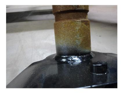
9. Also remove the paint from the reverse side of the motor mount plate to inspect the area where the through spigot of the steering pivot is welded to the reverse side of the plate as shown below. If there is cracking of the spigot to plate interface then this area should be ground and re-welded leaving a bead of weld above the surface of the plate
