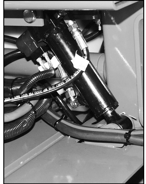
Figure 2-17: Depression Mechanism Cylinder
