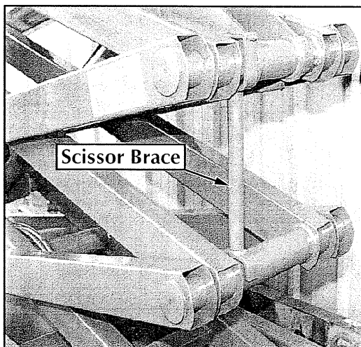
Figure 4-1: Blocking the Elevating Assembly
