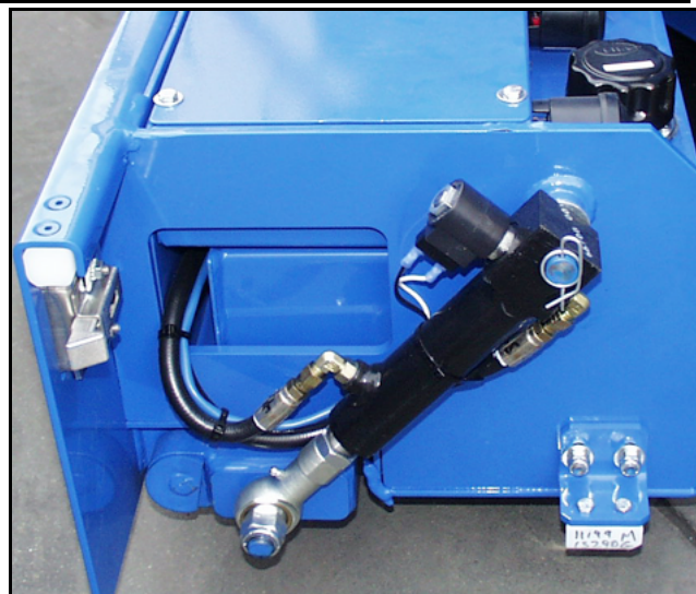
Figure 3-23: Depression Mechanism Cylinder
