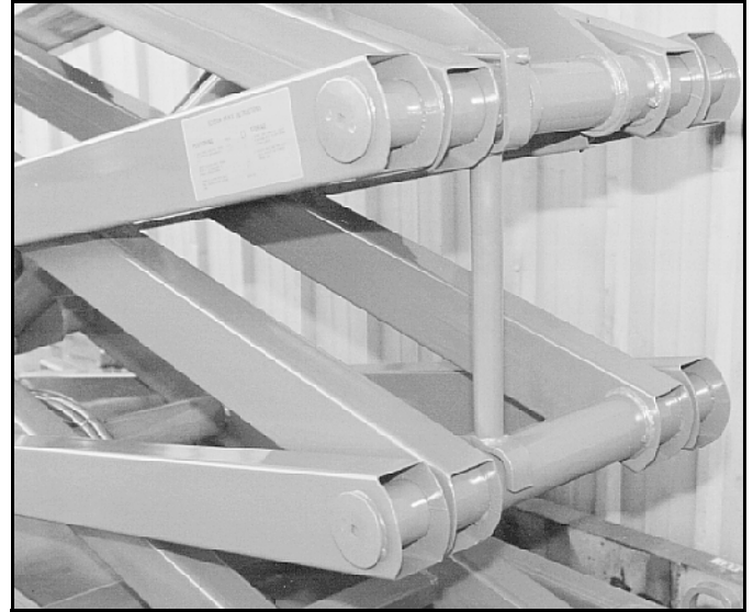
Figure 3-5: Blocking the Elevating Assembly--X20N, X20W, X26N
