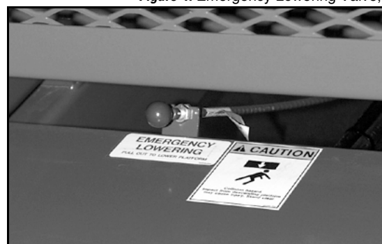
Figure 4: Emergency Lowering Valve,
