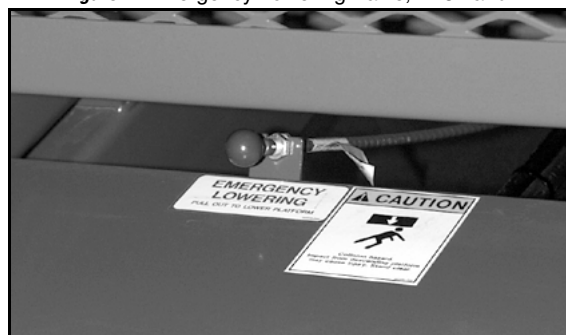
Figure 4: Emergency Lowering Valve, LX31 and LX41
