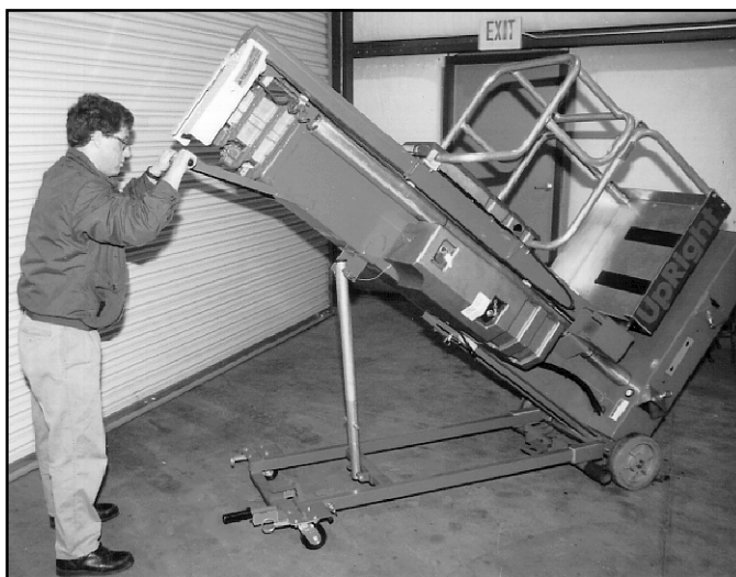
Figure 10: Compressing cylinder assembly
