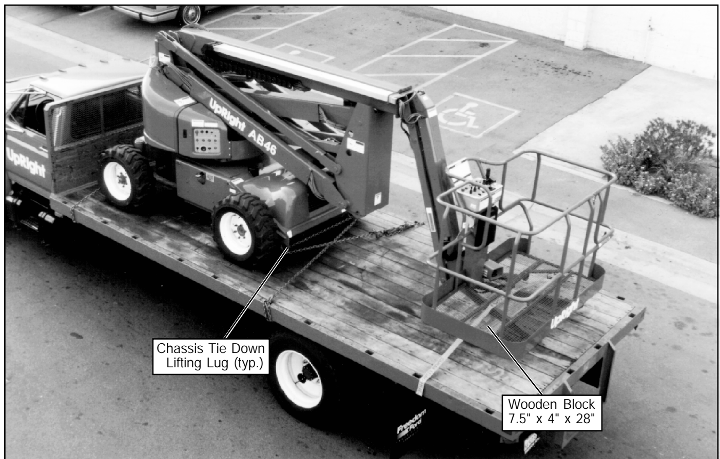
Figure 2-6: Securing the Machine for Transportation
