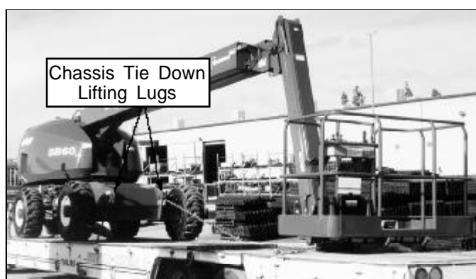
Figure 2-10: Rear chassis tie down lifting lugs.
