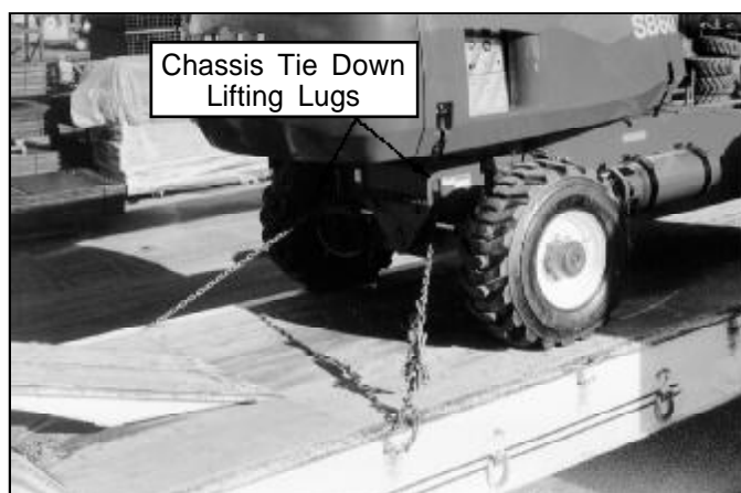
Figure 2-8: Front chassis tie down lifting lugs.
