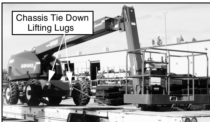
Figure 2-7: Rear chassis tie down lifting lugs
