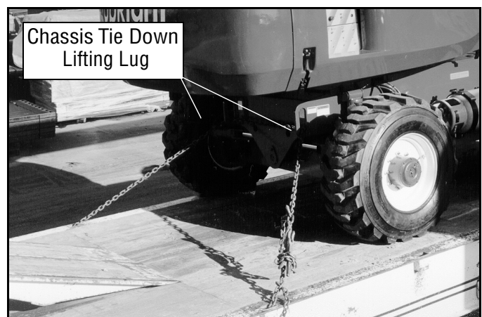
Figure 2-5: Front Chassis Tie Down Lifting Lugs
