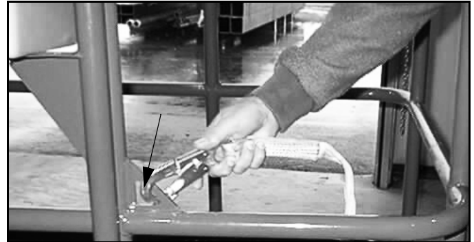
Figure 2-3: Typical Fall Restraint Anchorage Point
