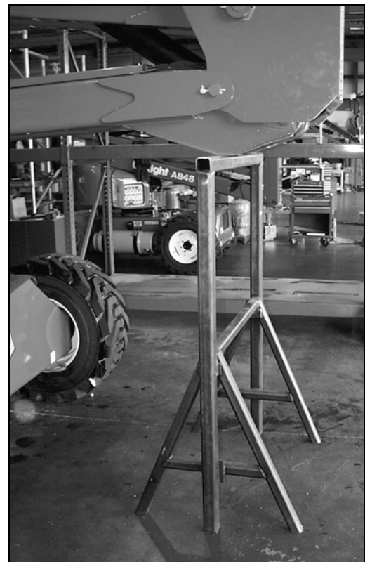
Figure 3-7: Elevating Assembly Brace
