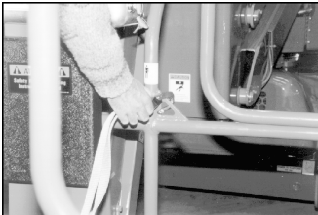
Figure 2-5: Typical Fall Restraint Anchorage Point
