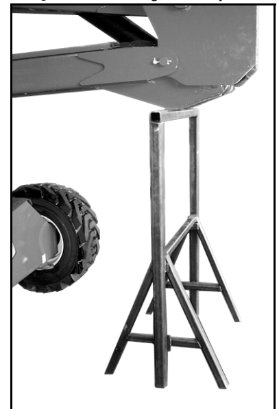
Figure 2-2: Elevating Assembly Brace
