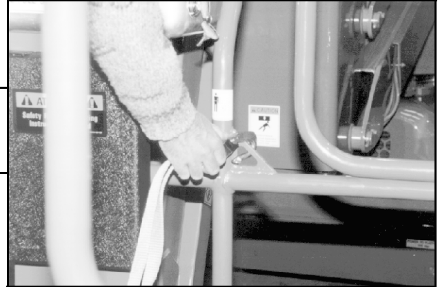
Figure 4: Typical Fall Restraint Anchorage Point
