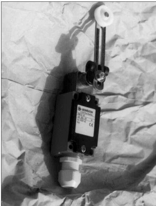
Figure 4-8: Boom Rest Limit Switch
