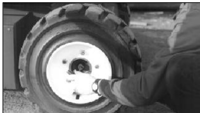
Figure 2-2 : Manual Brake Release
