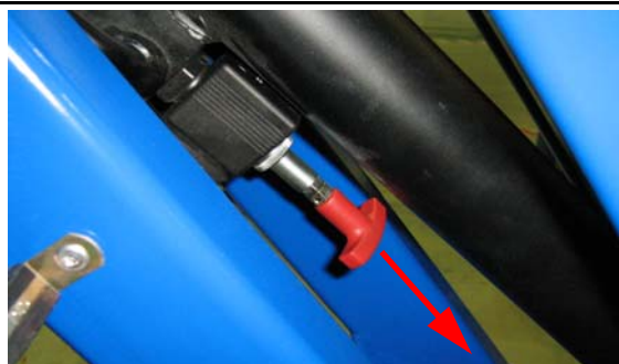
Figure 6: Emergency Lowering - Jib Valve
