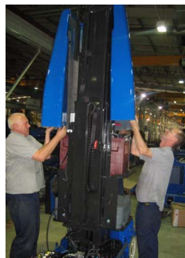
Figure 3-8: Mast Cover Removal
