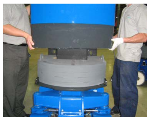
Figure 3-8: Mast Cover Removal
