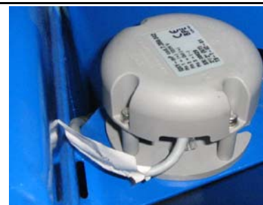
Figure 3-13: Tilt Sensor
