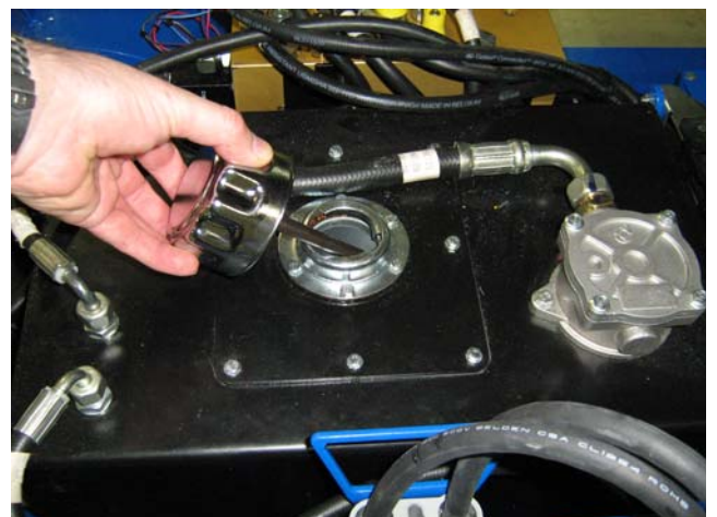
Figure 3-25: Hydraulic Tank Dip Stick
