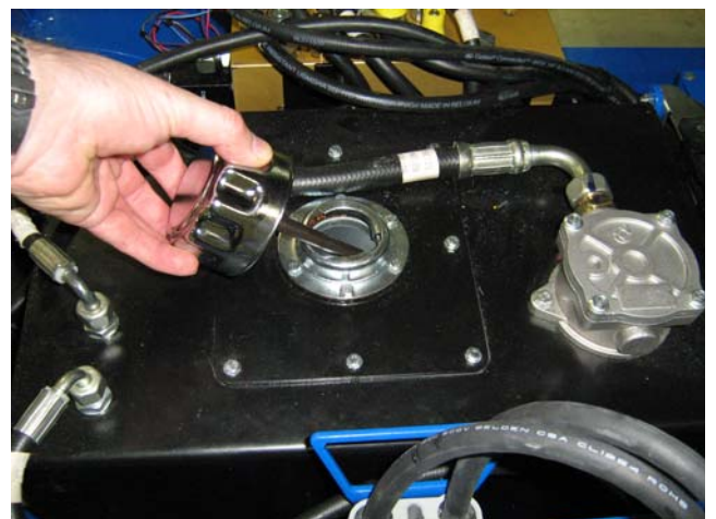
Figure 3-25: Hydraulic Tank Dip Stick
