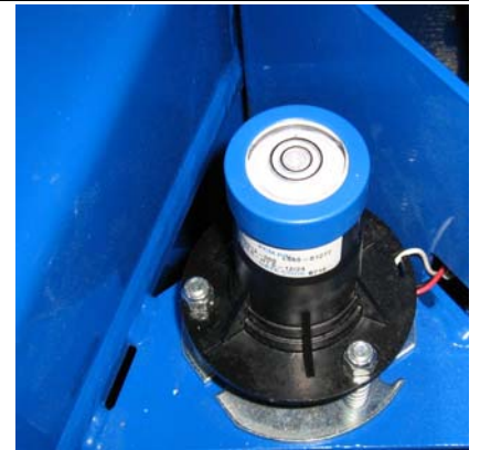
Figure 3-14: Tilt Sensor Spirit Level
