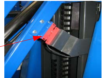
Figure 3-10: Boom Limit Switch
