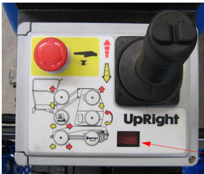
Figure 3-30: Upper Control Panel with Battery Indicator
