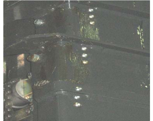
Figure 3-17: Wear Pad Retaining Screw
